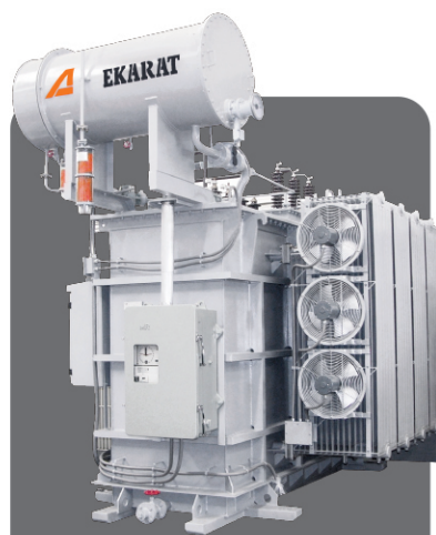
Conservator Transformer with On-Load Tap Changer, Cable Box and Force Air Fans
