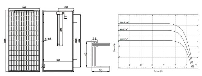
These data represent the performance of typical modules as measured at their out put terminals, and do not include the effect of such additional equipment as diodes or cables. The data are based on measurements made in accordance with ASTME 1036-85 corrected to SRC (Standard Reporting Conditions, also known as STC or Standard Test Condition), Which are:
