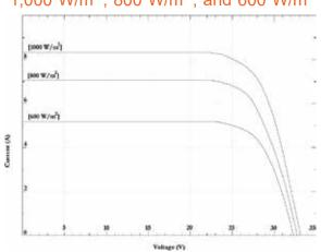
These data represent the performance of typical modules as measured at their out put terminals, and do not include the effect of such additional equipment as diodes or cables. The data are based on measurements made in accordance with ASTME1036-85 corrected to SRC (Standard Reporting Conditions, also known as STC or Standard Test Conditions), which are:
